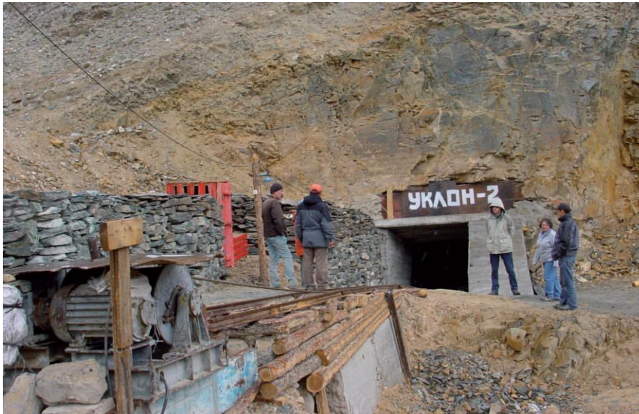
Inclined shaft at the Khovd Gol wolframite mine (Mongolia).
