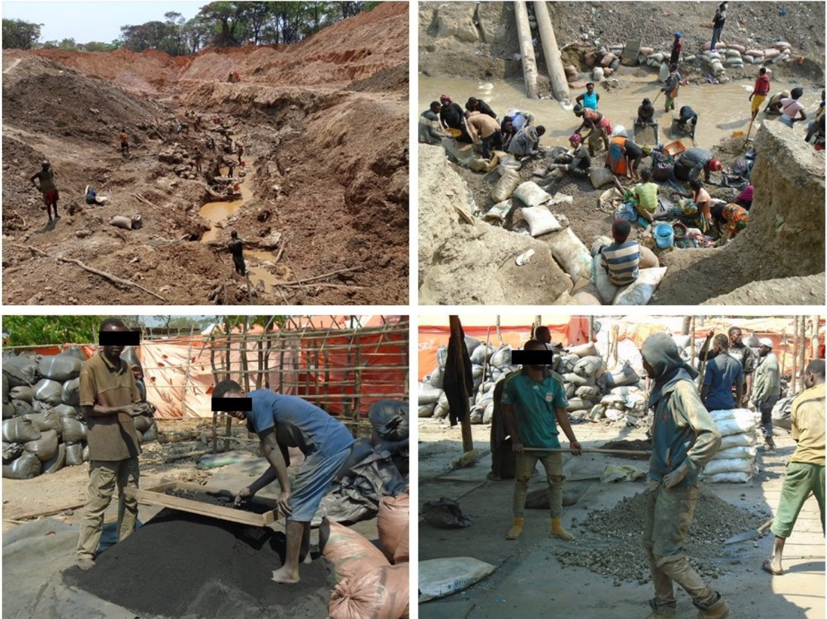
Figure 16. Processing methods in ASM. At the top left, lighter secondary particles are washed out of the ore in a washing trough. At the top right, ore is washed in a small stream. At the bottom left, ore is screened to remove coarse impurities. At the bottom right, crushed ore is filled into bags for transport.
