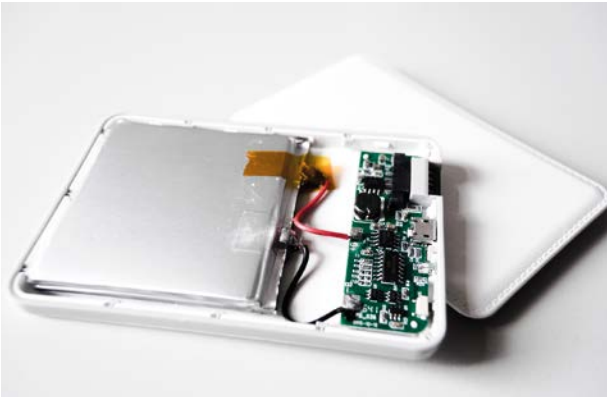
Fig. 3a: Pouch-Lithium-Ion Cell (Source: BGR).
