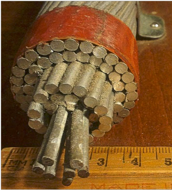
Abb. 3.90: Stahlverstärktes Aluminiumseil (Quelle: Clark Mills, Sample cross-section of high tension power (pylon) line.jpg, CC BY-SA 3.0)
