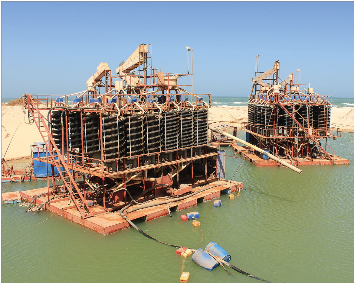
Figure 23: Floating wet mills of Mauritania Titanium Resources SA in Mauritania with the Atlantic Ocean in the background. Photo: BGR.
