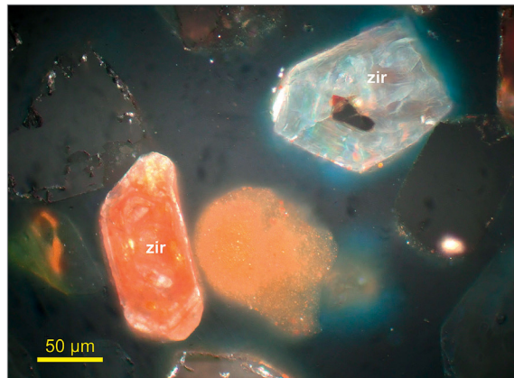
Fig. 10.16A: Section #16, RM, 500x, #: Different Zircons with inclusions and with disseminated Fe-phases.
