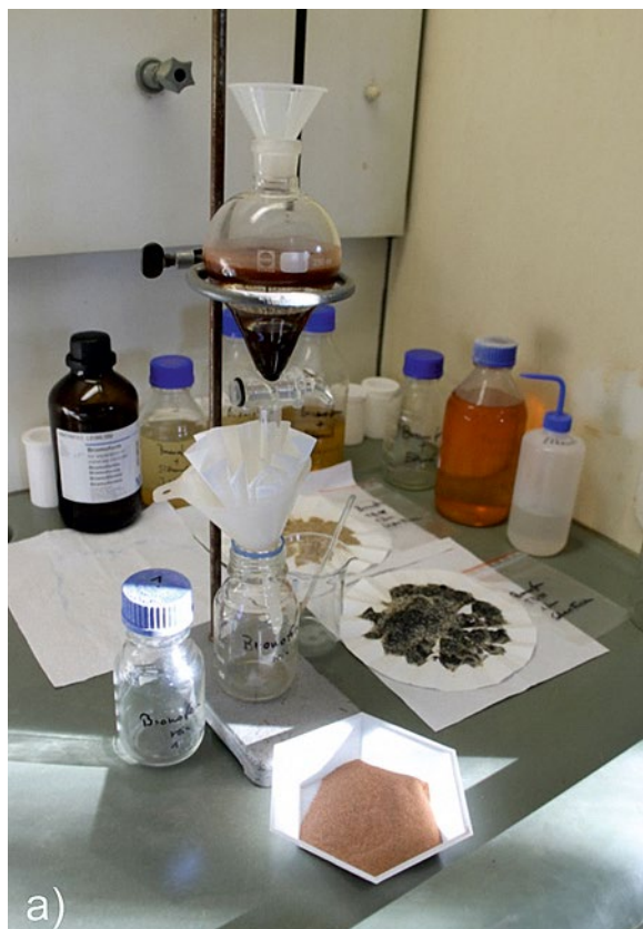
Fig. 6.9: a) Laboratory equipment for heavy liquid separation, b) Funnel with 200 ml \text{CHBr}_3 and stirrer.
