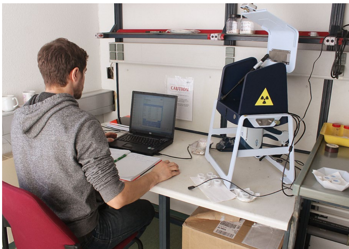
Fig. 6.13: Measuring station handheld XRF spectrometer S1 TITAN Model 800 – BRUKER.
