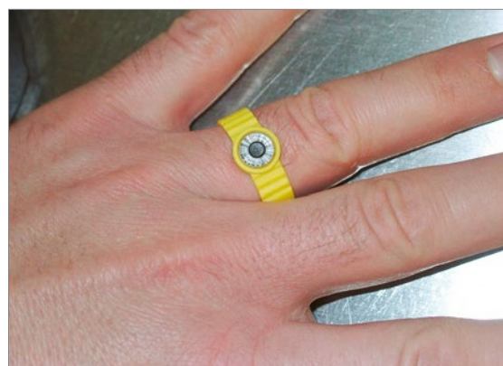
Fig. 6.71: Examination of the dose rate by finger dosimeter (thermoluminescence detector made of lithium fluoride– 1.0 mSv to 10.0 Sv) – HARSHAW BTKD (2001).
