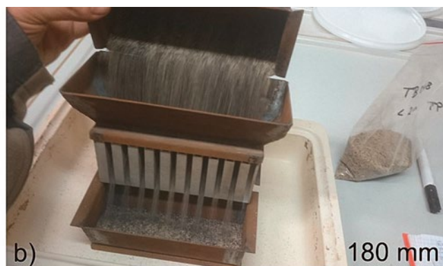
Fig. 6.8: Sample splitting with riffle splitter: a) 500 mm splitter for samples up to 100 kg, b) 180 mm splitter for samples up to 2 kg.
