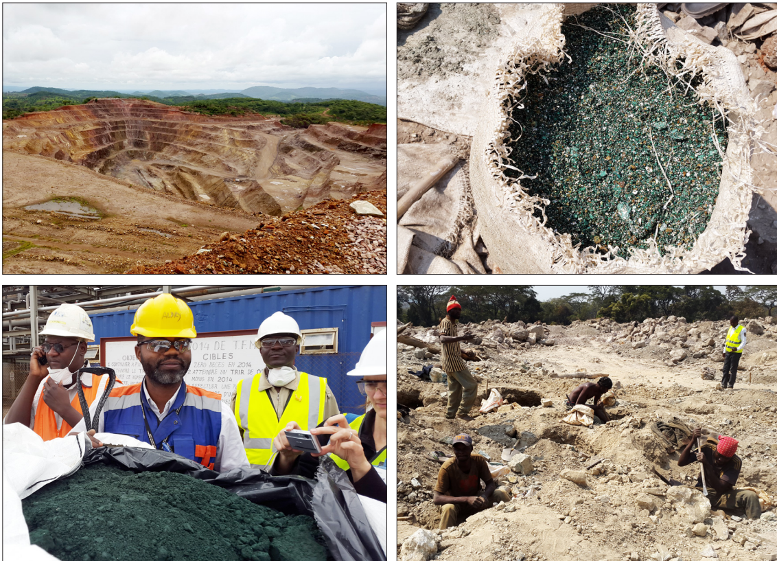
Figure 7: Industrial (left: Kwatebala Mine of Tenke Fungurume, Haut Katanga province) and artisanal (right: Kamwale Mine, Lualaba province) copper-cobalt mining in the DR Congo and its associated products cobalt hydroxid and cobalt-copper-concentrate (Pictures: BGR).
