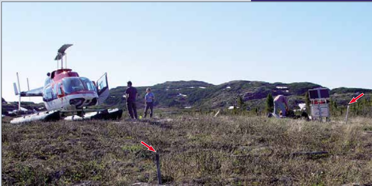
BGR field site in permafrost: pipes (marked by red arrows) emplaced in 2000 have risen above the soil surface by about 75 cm – evidence of a rapid drop in the land level.
