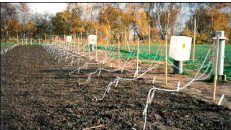
Monitoring site in the Fuhrberger Feld to measure groundwater recharge and nitrate leaching into the groundwater.
