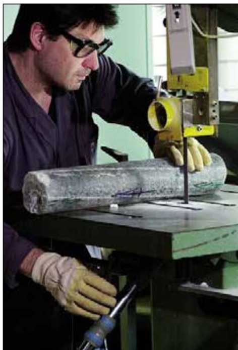
Specimen preparation, here sawing cores to length using a band saw.
