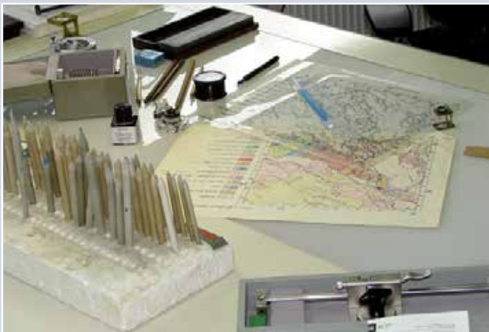
Above: Typical analogue cartographer's station. Drawing pens, retouching scraper, ink pots and whetstone are grouped around the drawing film. Beside them lie the hand-coloured map and colouring pencils.
