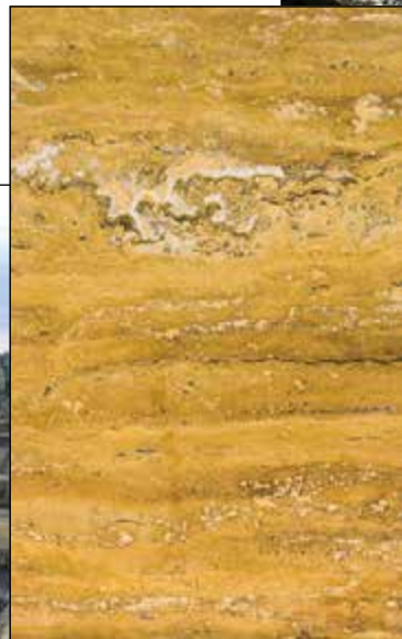
Travertine from Bad Canstatt is popular for the production of dimension stone slabs.
