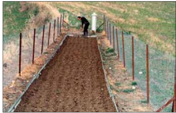
Standardized test plot for water erosion on Cyprus.
