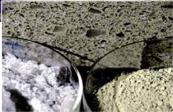
Crushed salt and bentonite before and after (in the dishes) compression in an oedometer test (above).
