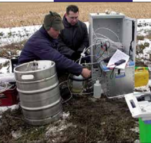
In the Fuhrberger Feld: sampling of groundwater from different depths using a multi level sampling well.
