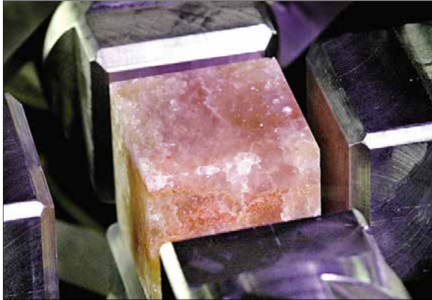
Rock salt specimen before creep testing in a triaxial test rig.
