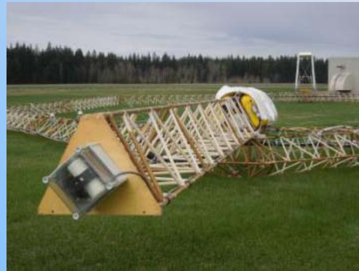
Mag sensor Readings at 45 Hz are taken in between each HM pulse
