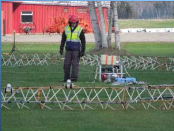
DGPS sensors on frame and base station
